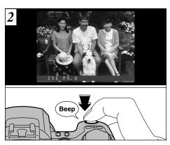
Position the AF frame over the subject and press the shutter button. The camera focuses on the subject in the frame and self-timer starts to run.
